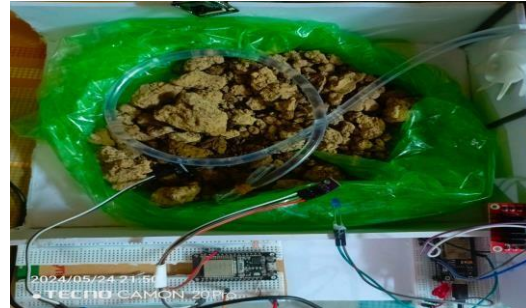
Figure 17 Connect the L298N and the sensor to ESP
