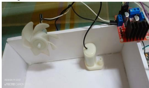
Figure 16 Connect the fan and pump to L298N
