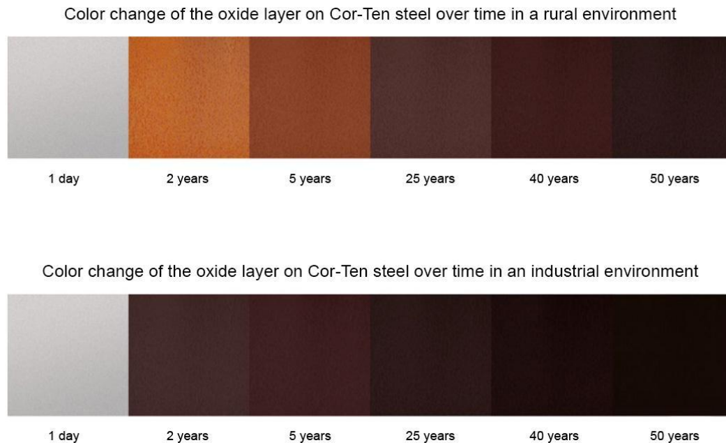
Fig. 19. Cor-Ten steel color change in industrial and rural environments
