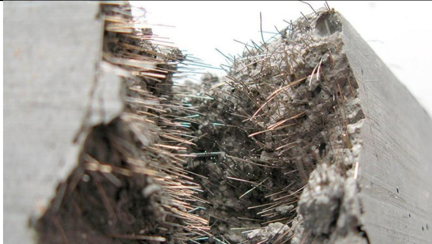
Fig. 12. Steel fiber distribution in the concrete matrix
