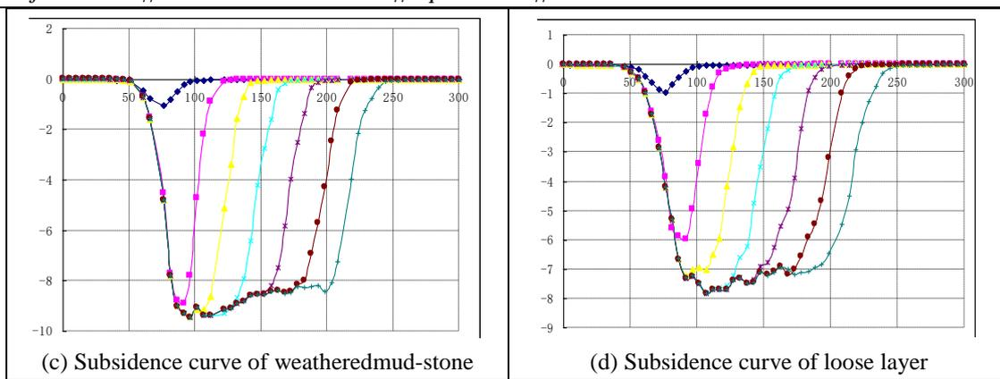
Figure 2 Dynamic subsidence curves of overlying strata at different levels
