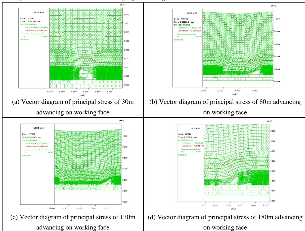
Figure 3 Principal stress vector diagram of different advancing distance of working face
