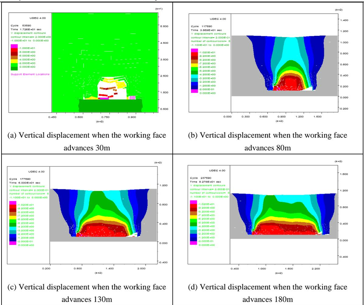
Figure 1 Vertical displacement diagram of different advancing distances of working face
