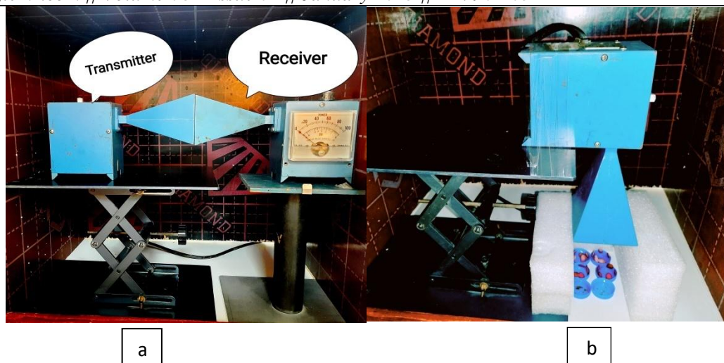
Figure 2: a-The horn antenna system used during calibration in the scientific laboratory b- Expose the seeds to microwave radiation
