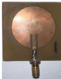
Figure 6: The top view of the fabricated microstrip circular patch antenna fixed with SMA connector
