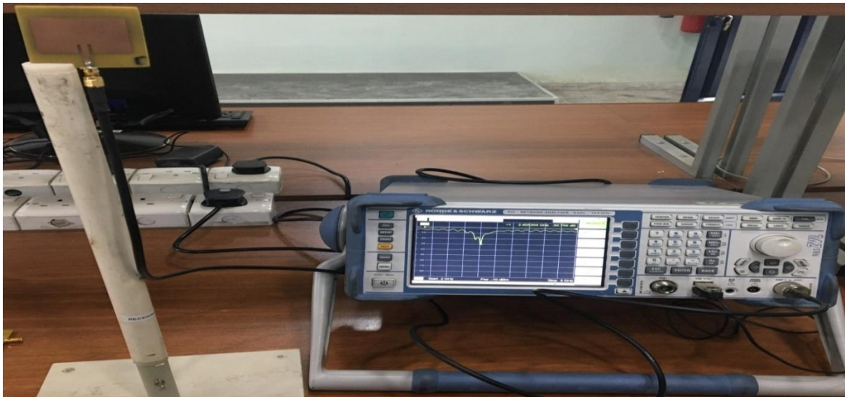
Fig. 8: Practical equipment set up using network analyzer for testing the fabricated rectangular patch antenna.
