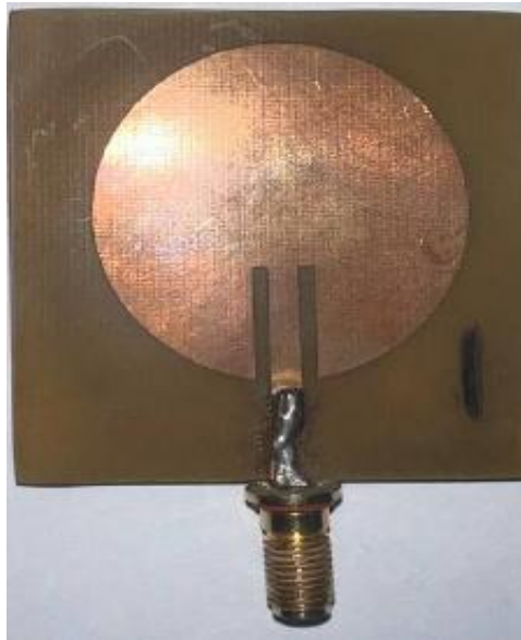
Fig. 3. The top view of the fabricated Microstrip circular patch antenna fixed with SMA connector
