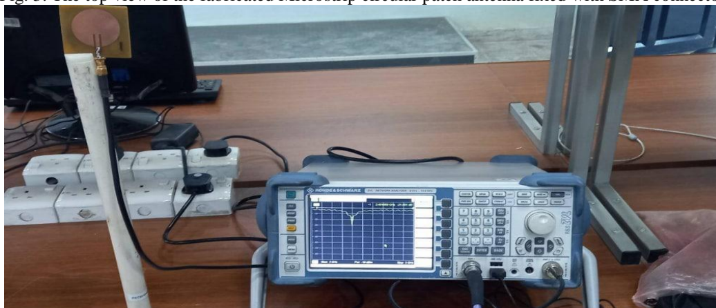
Fig. 4. Practical equipment set up using network analyzer for testing the fabricated circular patch antenna.
