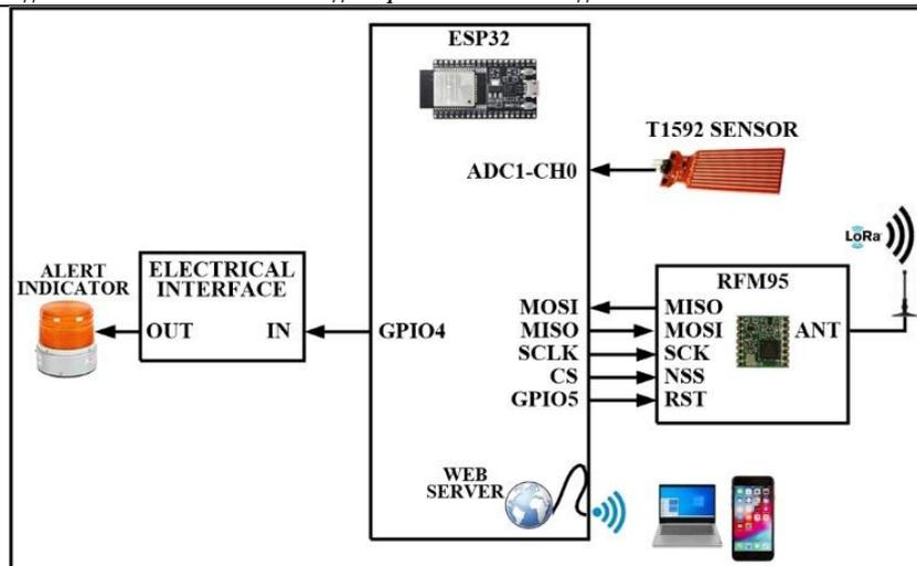
Figure2. Terminal nodes architecture.
