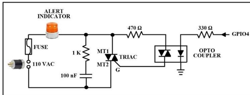
Figure3. Alert indicator electrical interface.
