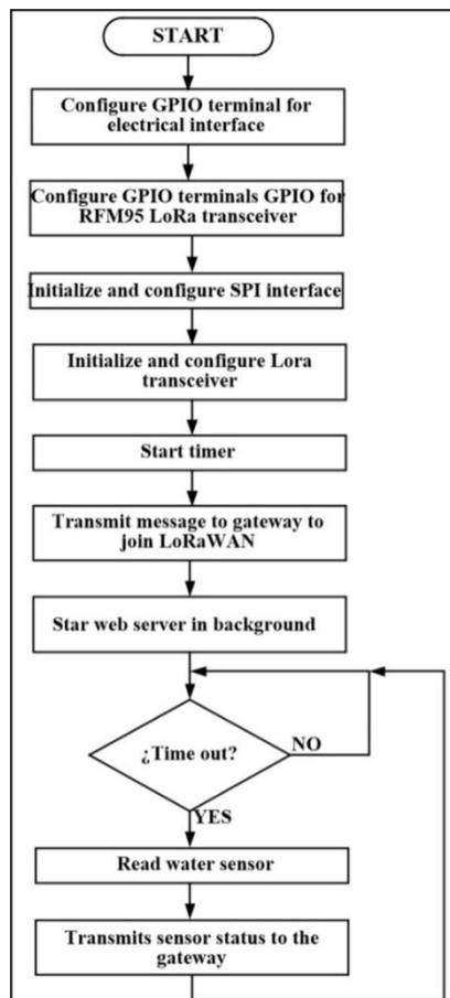
Figure4. Terminal node program flow chart
