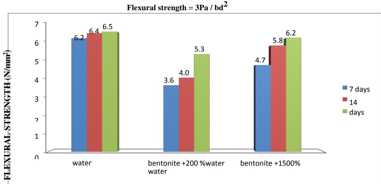
Fig 6. FLEXURAL STRENGTH OF CONCRETE
