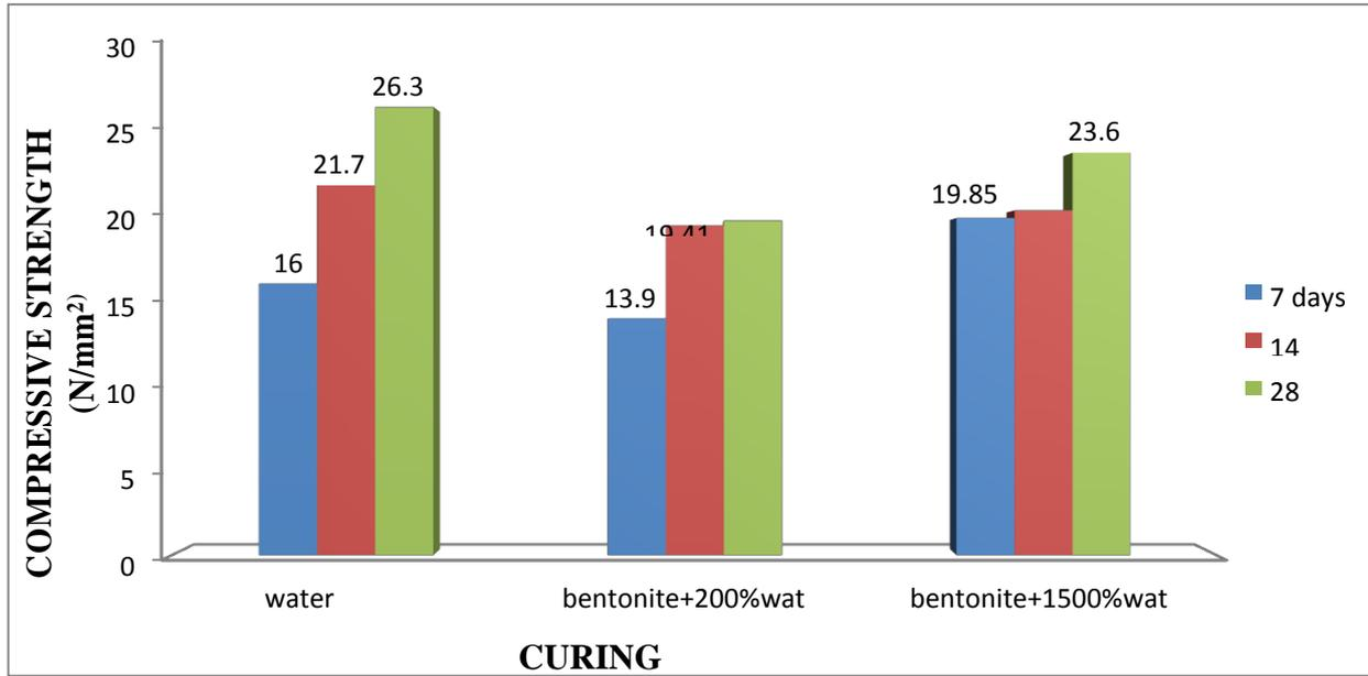
Fig 4. COMPRESSIVE STRENGTH OF CONCRETE
