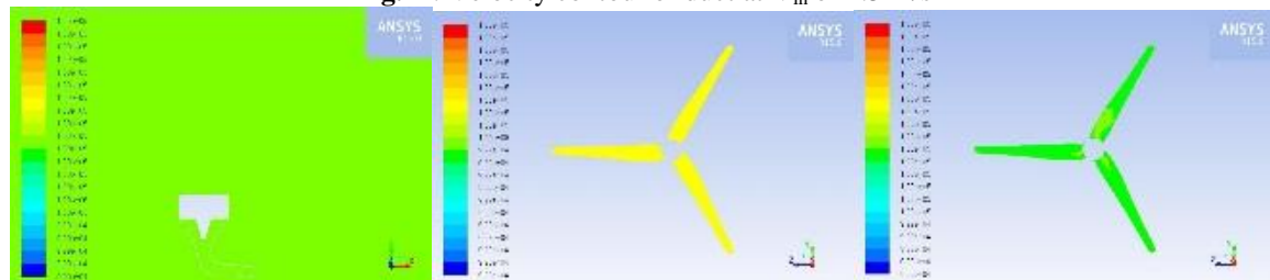
Fig.12: Pressure contour of duct & blade at V_{in} of 2.5 m/s
