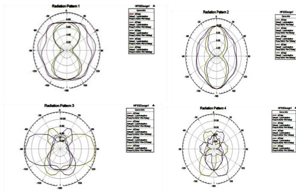
Figure 10: Plot of Radiation Pattern at 2.4 GHz, 3 GHz, 5.2 GHz and 5.8 GHz
