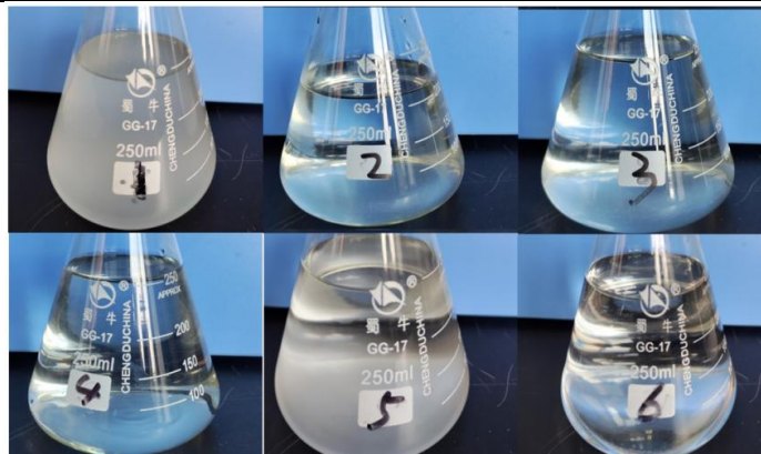
Figure 11: Photographs of Specimens after Heating (No. 1–4: Four different scale inhibitors; No. 5–6: Blank groups)
