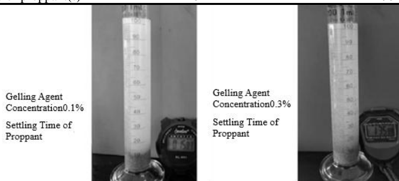
Figure 8: Proppant Carrying Capacity of Slickwater with Different Functional Dry Powders
