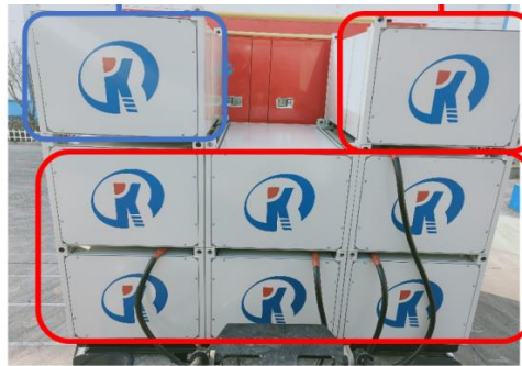
Figure 2: Actual Photo of the Modular Unit of the Vehicle-Mounted Remote Fire Extinguishing Device
