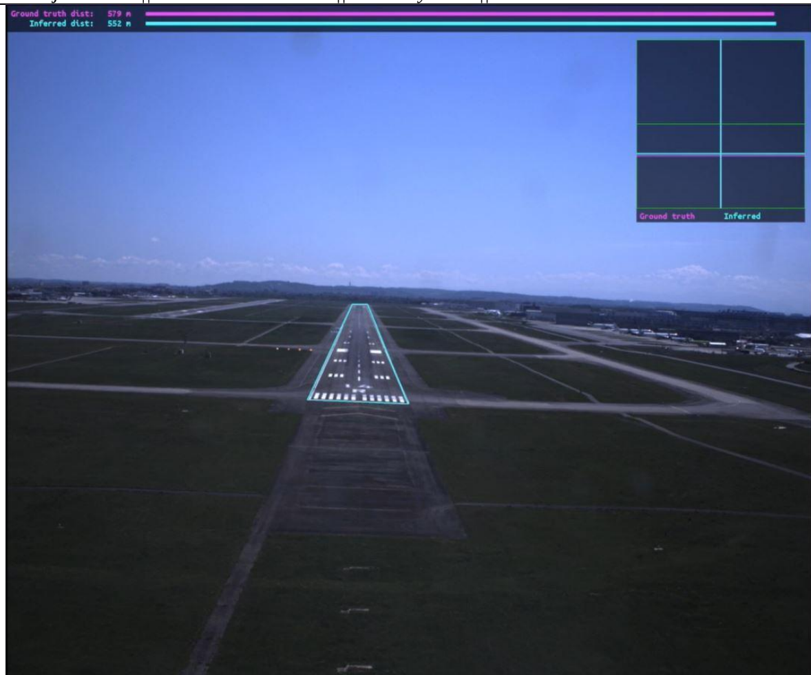
Fig.2. The Wayfinder computer vision software detects the runway [11].
