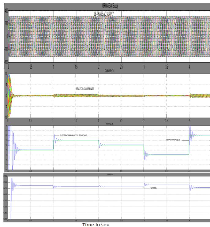
Figs.7 Simulation results for 18-phase machine for different load conditions
