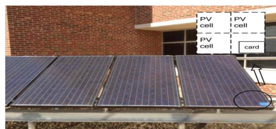
Fig. 16. PV panels of phase a : One cell of the third panel is partly covered.
