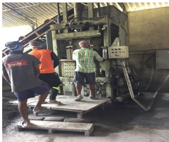
Production of concrete blocks using Dual compression machine
