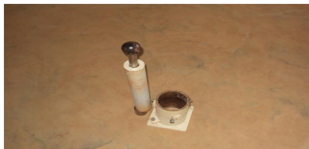
FIG 3. Proctor Compaction Test
