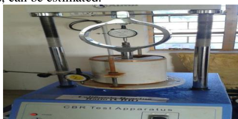
FIG 4. Californian Bearing Ratio test
